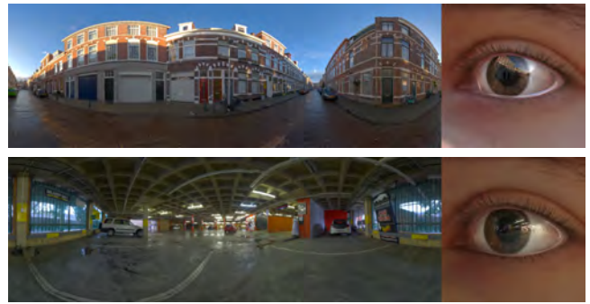
Figure 10: We use HDR panoramic images for reflections and ambient light in the scene. Here you can see two example equi-rectangular panoramas, with example eye renderings.
