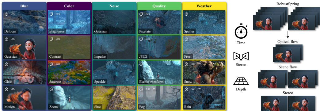
Figure 1: RobustSpring is a novel image corruption benchmark for optical flow, scene flow, and stereo. It evaluates 20 image corruptions including blurs, color changes, noises, quality degradations, and weather, applied to stereo video data from Spring. For comprehensive robustness evaluations, RobustSpring’s image corruptions are integrated in time, stereo, and depth, where applicable.
